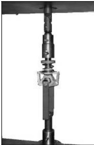
**Figure 5** Experimental setup for traction tests on the INSTRON machine.
